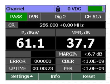
The IT-19C can measure signal levels of both analog and digital channels. For analog signals the meter will display the video carrier level, video frequency, C/N, and V/A ratio. For digital channels, the IT-19C measures the digital average channel power and displays the center frequency.
